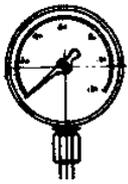
This gauge indicates the steam pressure inside the boiler in pounds per square inch.
